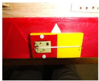
that can be seen just above and to the left of the lower 2-56 bolt head. The small vertical wire just to the right of the peg becomes energized and burns through the DT band at the pre-programmed time. The pin (on the right) was used to make this photograph only. On a functioning airplane a line would extend from the rubber band to the stab, first to hold the trailing edge down and then to release it after the DT band has been burnt through.
