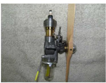
This Bill Schmidt's latest project, a first model Atom – 0.9 displacement ignition engine – ask how he makes it so pretty! Notice that plating!
