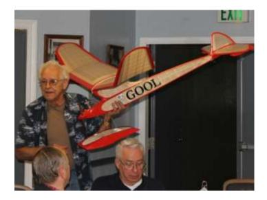
Nick brought two Gool models in the 7 foot size to show us. The flying surfaces are covered in silkspan and the fuselage is covered in silk.
