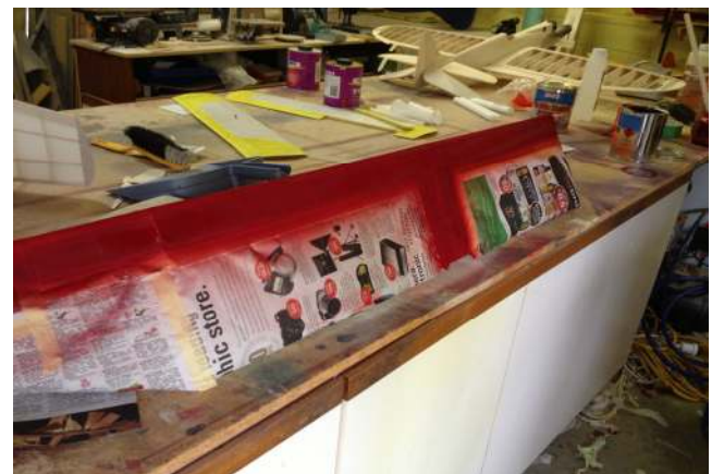
Two coats of coloured dope sprayed onto white polyspan.
