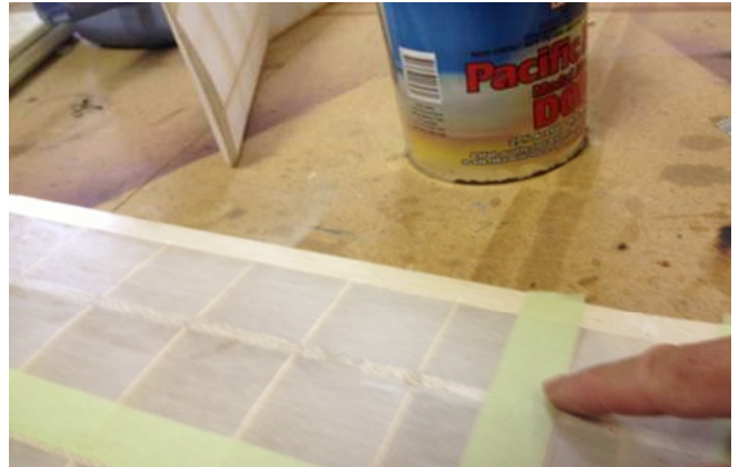
Seal masking tape with a smear of clear dope to ensure the colour doesn't creep under the tape.
