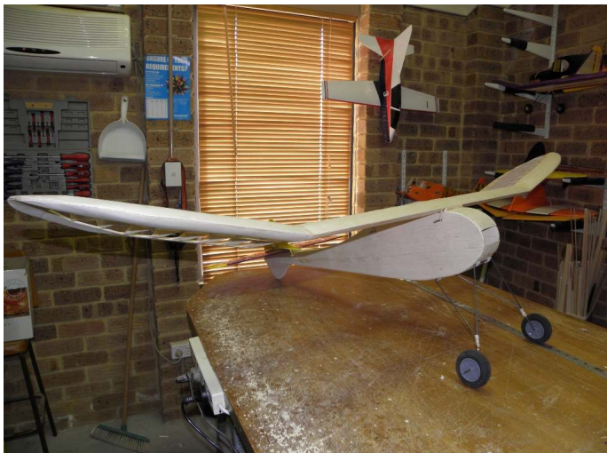
Fuselage – port side view. Thin but deep fuselage with plenty of room for R/C.
