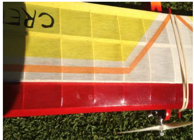
The finished product after being fuel proofed with clear
