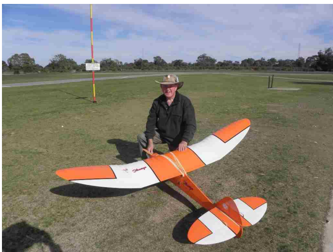
Flamingo Has Turnigy C3548-800 KV motor, 60 Amp Turnigy ESC, Split Wing, Removable U/C $300 Empty $400 Full
