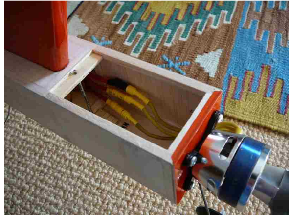
Plenty of room for the battery – helps with C.O.G.
