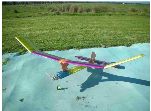
Ray 'Hi-Ho' Silbereisen's Electric Zoot Suit. Flight testing was successful and the aircraft is stable in climb and glide. Weight is comparable to its FF progenitor..
