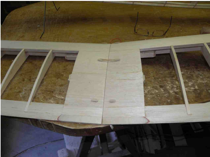
Wing retainer system using two hooks and lacky bands..
