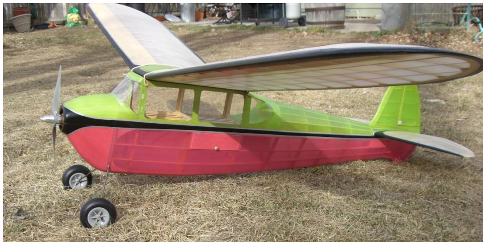
This view shows the classic lines. Side windows are clear Monokote. You can see the battery access hatch on the side.
