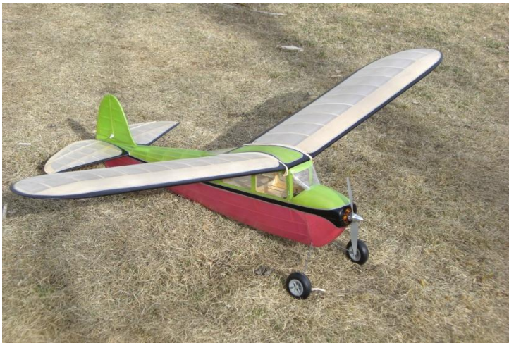
Brushless motor and speed control- roughly a .30 glow equivalent.
