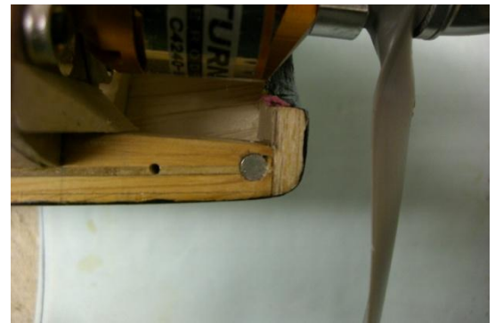
Cowl is held on with dowel pins and small magnets.
