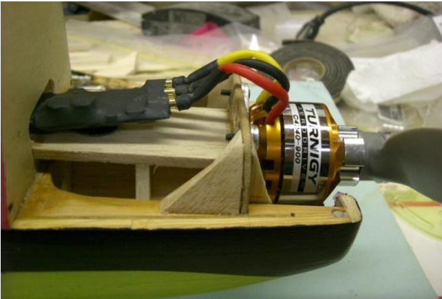
Brushless motor and speed control- roughly a .30 glow equivalent.
