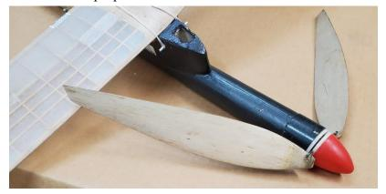
catch the top of wing and finish up in this position while the lower blade hangs limply in the wind. The result is at best a poor glide, and may even cause the plane to spin in.
