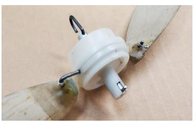
engage a hole in the hub to effect an instantaneous stop. The blades fold back under the wing every time. A variation on this theme is called a reverse Montreal; instead of a separate pin, the entire prop assembly moves forward to release the stop pin and is held there by the torque. When the torque decays the prop assembly is released and moves back allowing the integral stop pin to engage the hole in the hub.
