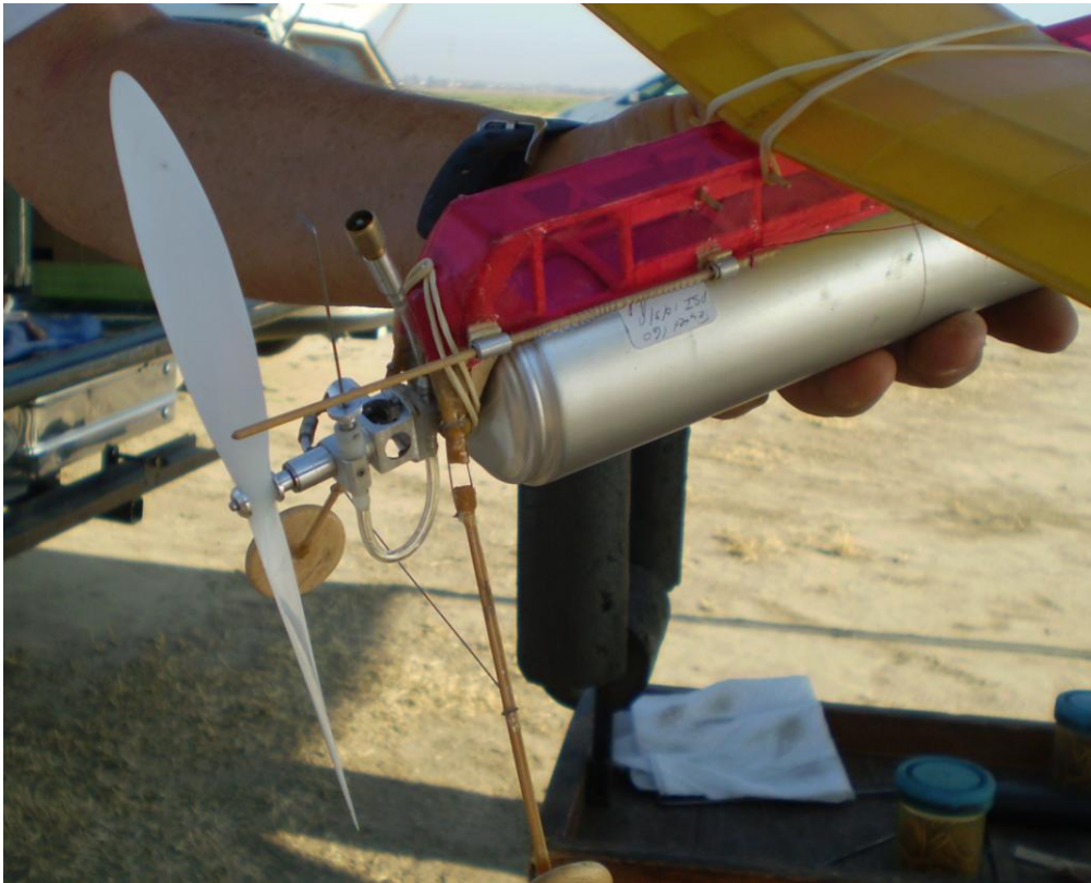
The neat prop brake on Hal's design-prevents the motor from pulling vacuum on the tank after rundown
