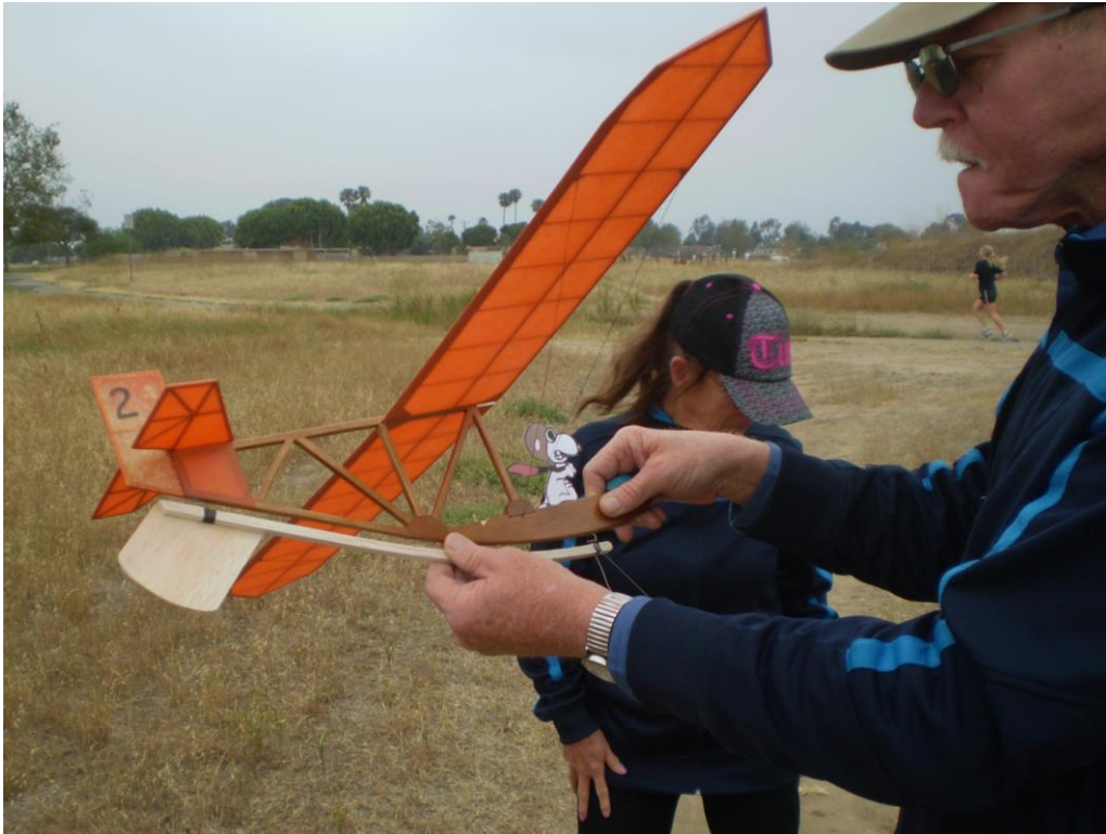
Randy installing the towing sub-rudder required to have a chance at success with this launch technique-note the complete lack of interest of the observer in the far background-typical
