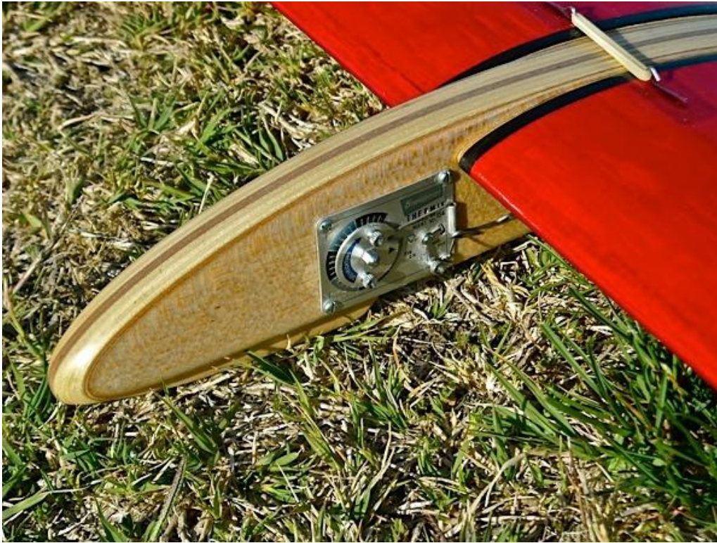
Pod and timer installation on the Dragmaster -so clean and simple
