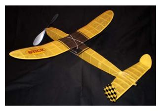
and Esaki covering. Builder supplies the timer, adhesives and finishing materials. The model is targeted to those who may want to try higher performance rubber powered models and don't want to build the traditional size old timer designs, or don't want to deal with the modifications required to add D/T function, etc. There is a page or two dedicated to the Yardstick at www.cbmodeldesigns.com if you wish to investigate further.
