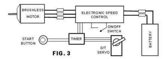
The connections between the battery and the ESC need to be capable of passing high current without significant losses. The motor leads need to be kept as short as practical and good connectors used again to minimize losses. It's a good idea to make the battery removable from the plane for charging.
