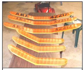
My Twin Pusher wings and stabs - lightweight Polyspan covering
