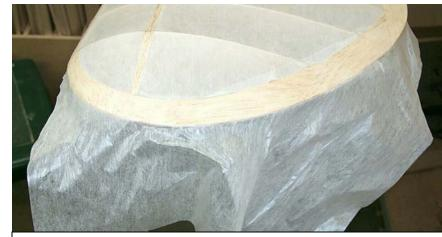
Same tip on ½ A Texaco Powerhouse after all the wrinkles were shrunk out and stuck down. Works great and no need for a splice to get around the tip!
