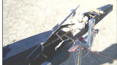
The motor let go as Bernie was inserting the propeller on this Joe Williams Moffett after winding and after removing the blast tube
