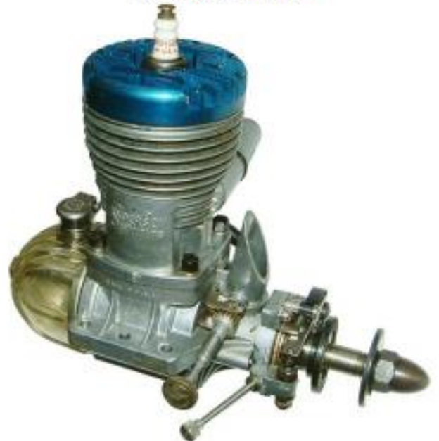
Anderson Spitfire .65 Spark - with high compression head
