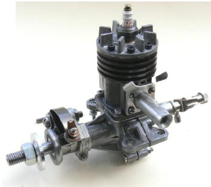
The finished GHQ, after replacement of the timer assembly. The cast timer assembly frame cracked and failed during an early flight of the Finneran Flyer, causing an instant lack of power when the engine timing changed. Below is the Finneran Flyer, the handiwork of Albert Fisher.
