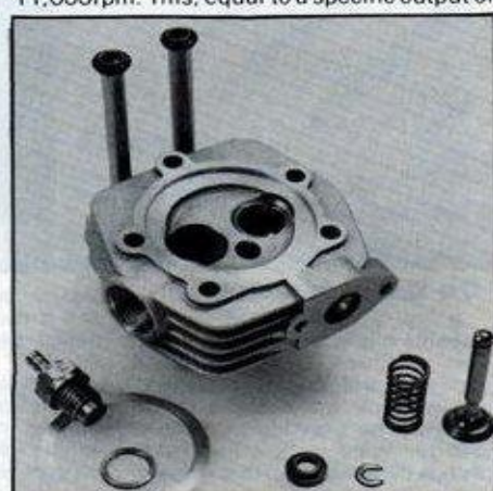
Left: FS-40 with rocker box cover removed. Sturdy rockers are same as on FS-60 and FT-120, and right, the FS-40 cylinder head showing inlet valve assembly removed.
