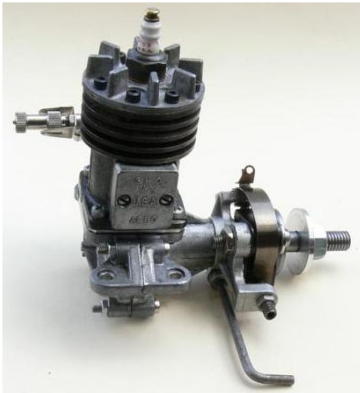
The finished GHQ, after replacement of the timer assembly. The cast timer assembly frame cracked and failed during an early flight of the Finneran Flyer, causing an instant lack of power when the engine timing changed. Below is the Finneran Flyer, the handiwork of Albert Fisher.
