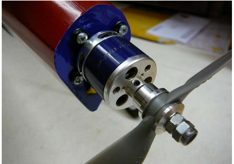
The Hyperion Z2213-24 on my 1/2A Stardust Special was originally used with a 3S pack but now works well with a 2S pack by using a larger prop -see text.
