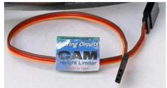
The CAM height limiter is small and light. It fits between the ESC and Rx to automatically cut the motor at a set height.
