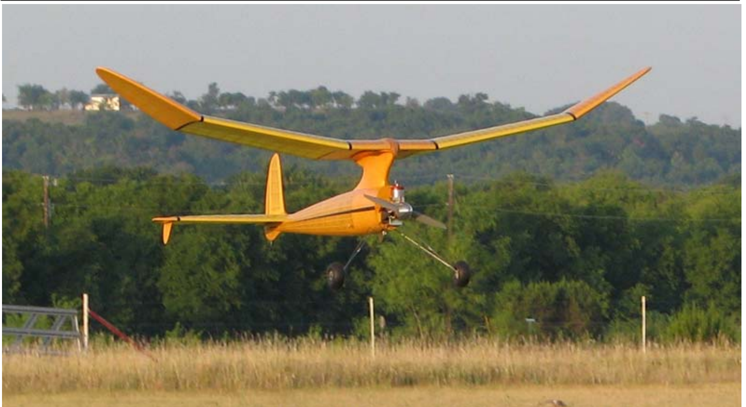
Tandy Walker's Goldberg Sailplane approaches for landing on an early test/trim flight. Power is McCoy 60 Series 20 on spark. Engine cowl is still to be fitted. One of the Master Builders.
