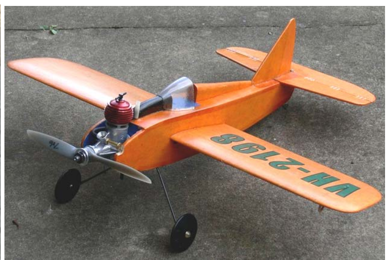
Above: David Owen's new TP2.5 Diesel test engines fitted to his Sabre Trainer. It is reported to be running very well and hauls the ST around in excess of 80mph. Model was flown at the 2010 Vetrans' Gathering
