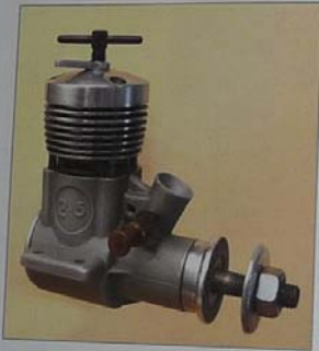
Second Mk 7 variant has sand blasted crankcase and no anodising.
