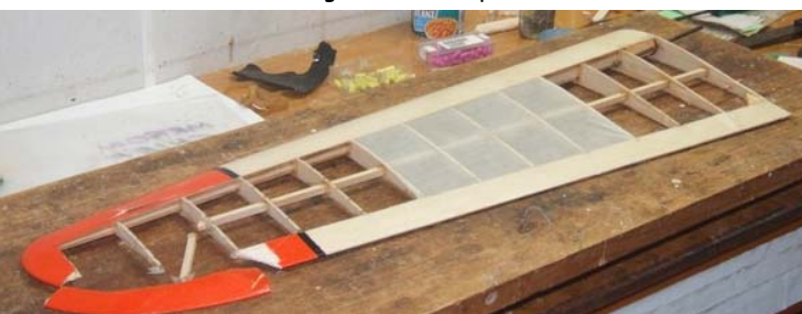
Left hand wing panel only sustained minimal damage.
