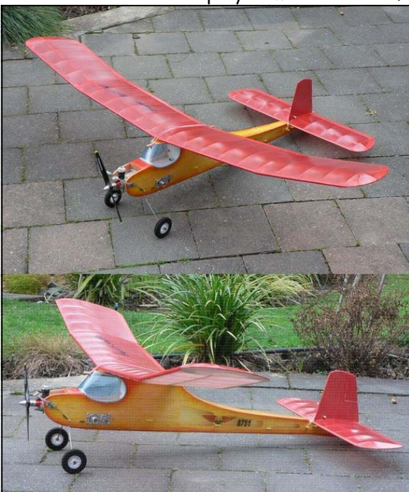
48" Super Sniffer. All covered with tissue and dope but main wing was first covered in laminating film.
