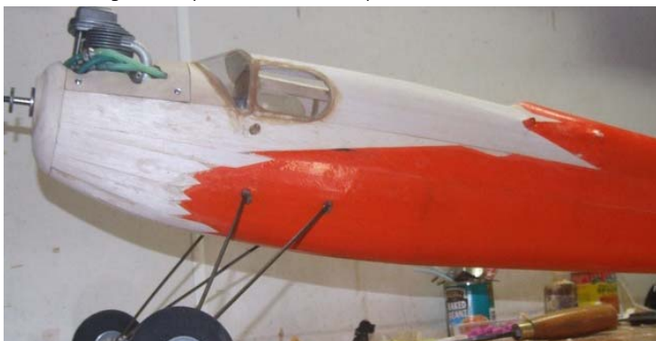
Fuselage structural repairs complete - every plank on bottom of Fuselage had to be spliced.
