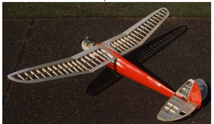
Structural repairs complete, covering still to be completed.
