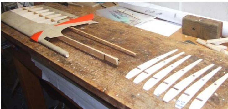
Wing centre panel after broken parts had been removed.
