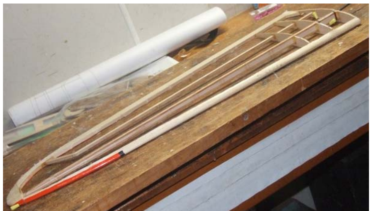
All that remained of the RH wing panel after shattered parts were removed. Almost every rib had to be renewed.
