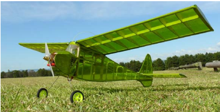
Pieter's Tomboy: 200g AUV - an exercise in lightweight construction and fitting - flies on only 2A from a 2S 350 mAh LiPo
