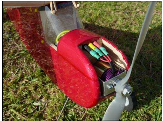
Front end of Lou's Tomboy was built using the longer nose shown on the Aeromodeller plan. A new firewall was added 2 cm in front of F1 to serve as a battery compartment. No lead was required to balance the model
