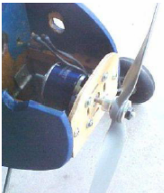
Electric Motor installed on ply mount plate and screwed to front of existing bearers
