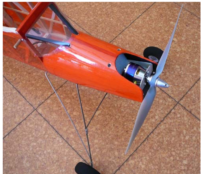
A light, compact motor such as the Hyperion 3013-16 (110g) is all that is needed for moderately sized Texaco model.
