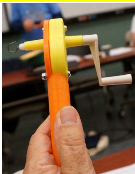
Simple rubber motor winder.
