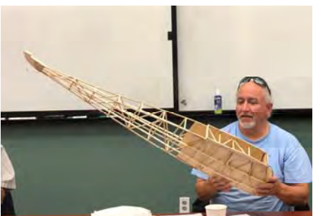
Ken Martinez: one design Clipper fuselage, 3/16" x 1/8" strips, sheeted front, wire wing rubber hold downs.
