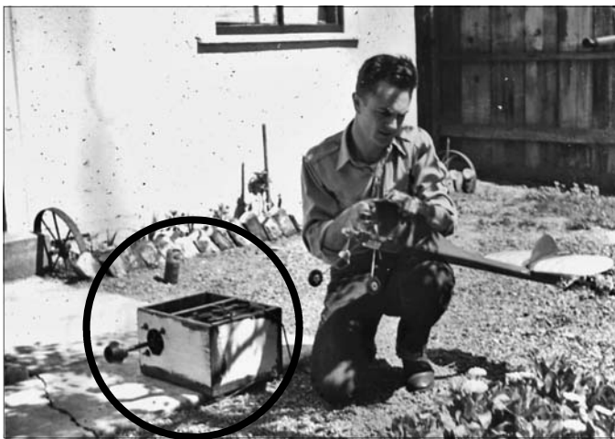
Above: Dr. Volponi tunes up his Class B Westerner using his 'state of the art' starter, featuring a full size, 6v automotive battery and a rather long extension shaft on the automotive starter motor
