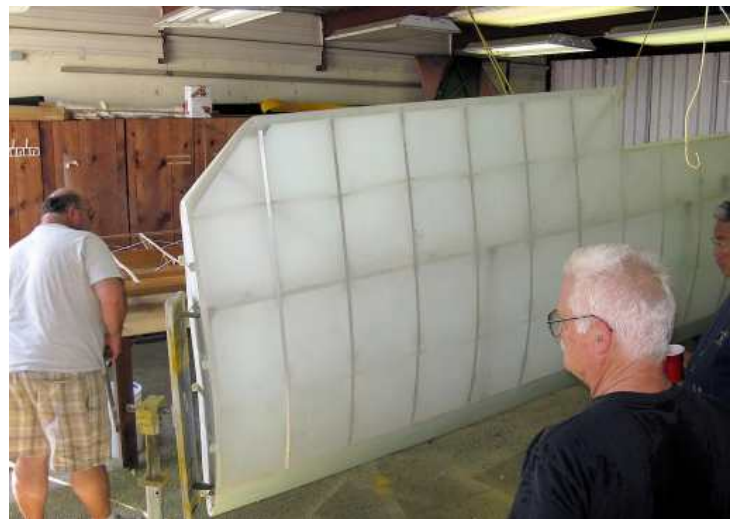
The undamaged left Pietenpol wing was recovered at a workshop last fall. The new right wing awaits better weather for covering.
