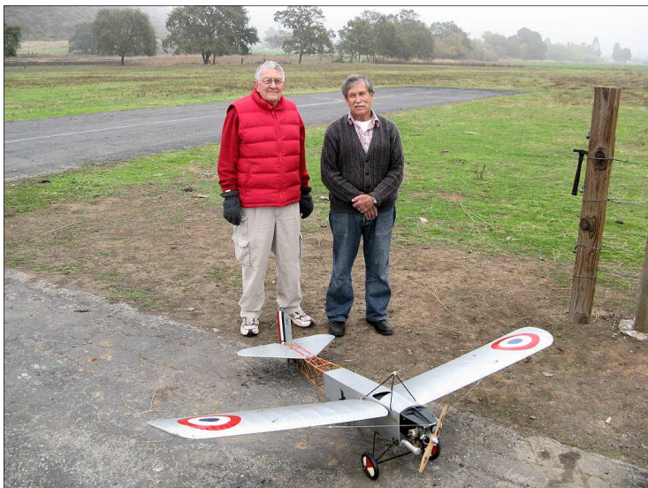
Henry Smith built this Lou Procter Antic some years ago and recently passed it on to David Saso. Glow powered, it flies magnificently, sez David. Note the flying wire braced wing panels...
