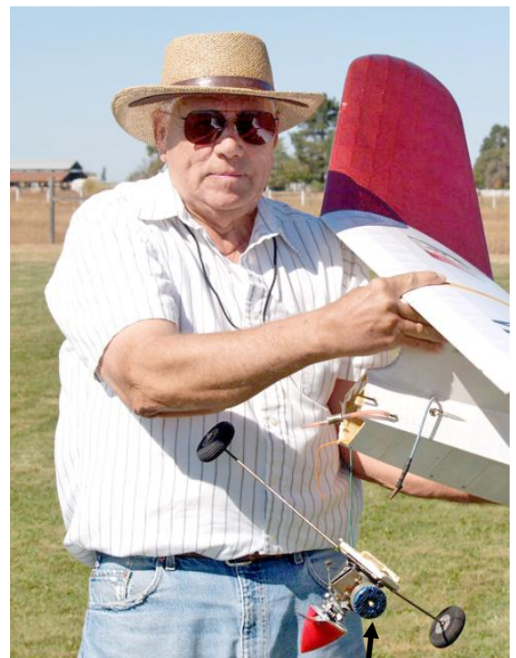
Above: Wayne Conner wasn't so lucky last year. He couldn't figure out why he got a short engine run and was having a hard time trimming the glide portion of his flight. Turned out that his CG had moved aft considerably after the engine/firewall fell off stopping the engine. Stop buying that cheap glue Wayne!
