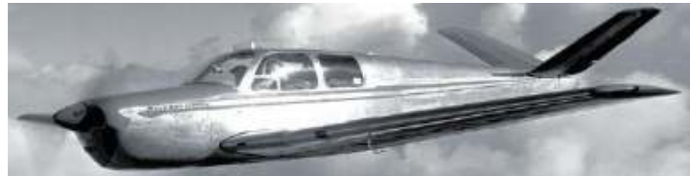
While Beech's Model 34 was not a success, the Model 35 Bonanza certainly was. One thing the Bonanza had in common with the Twin Quad was the distinctive V tail. The airplane is still in production (and also
