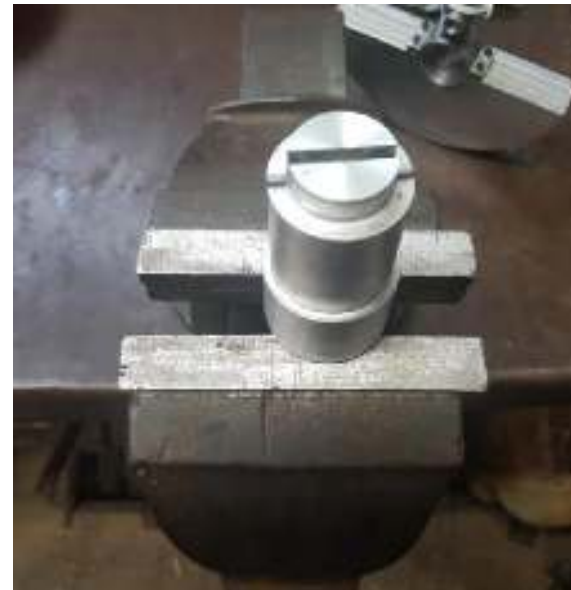
Above: Showing the tool for unscrewing the back plate. Below: Gudgeon pin removal tool.
