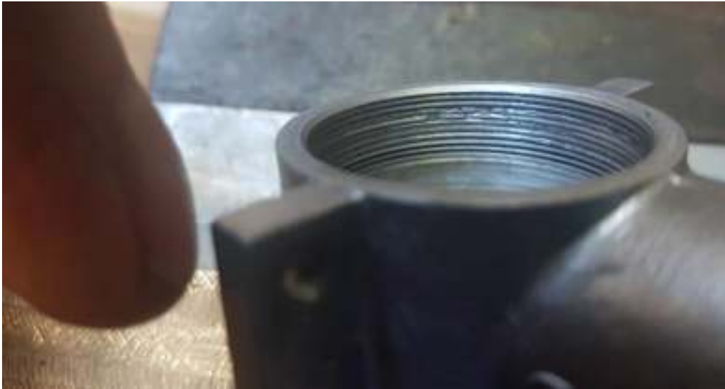
Above: Showing the crankcase galling.
