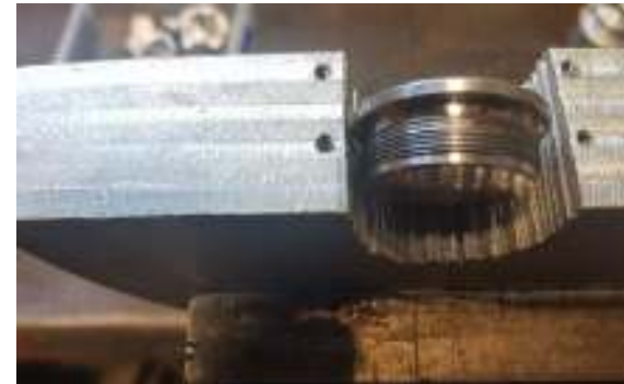
Above: Showing the back plate galling.
