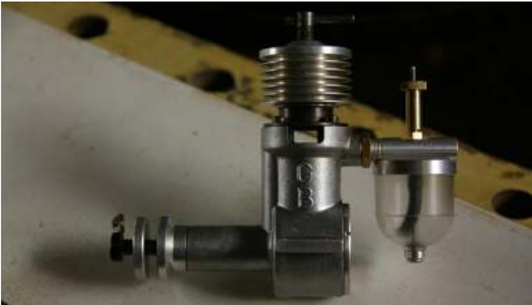
Opposite side view of my engine complete with new carburettor.
