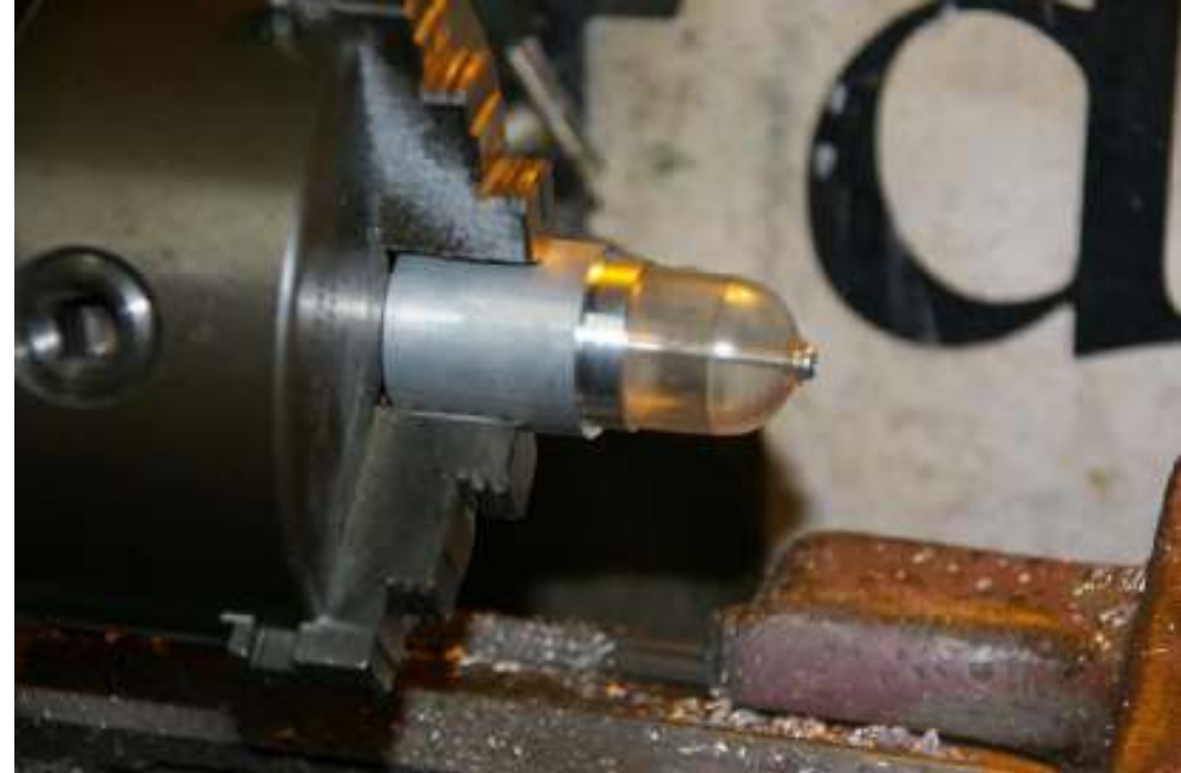
Showing the fixture for machining the outside hemisphere of the tank.
