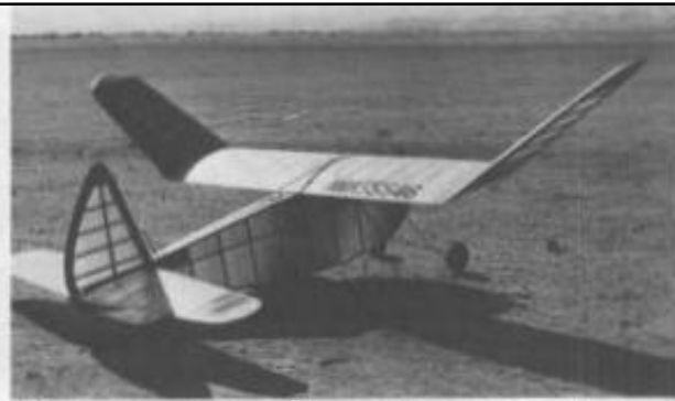
What could be a better combination? Ultra simple to build, and ultra stable to fly. Note DT. Fin goes into slot when popped up.
