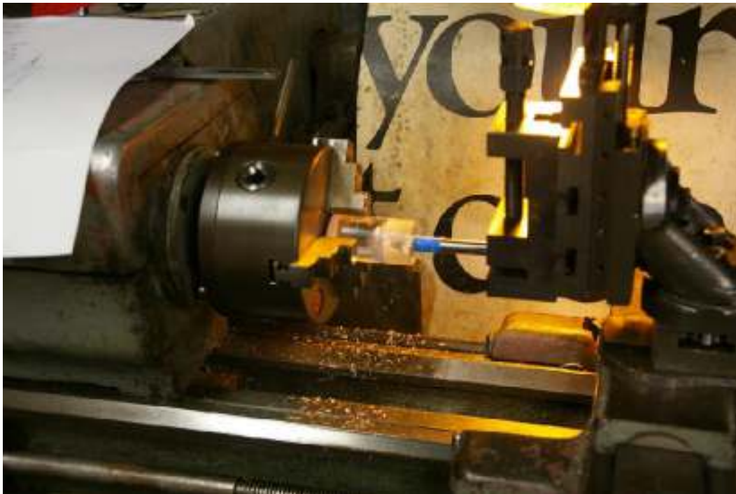
The machining of the 1" hemisphere with a router cutter.
