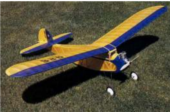
Bob Munn's 84-inch-span Powerhouse is covered in yellow and blue silk, and uses an O.S. .61 four stroke engine.
