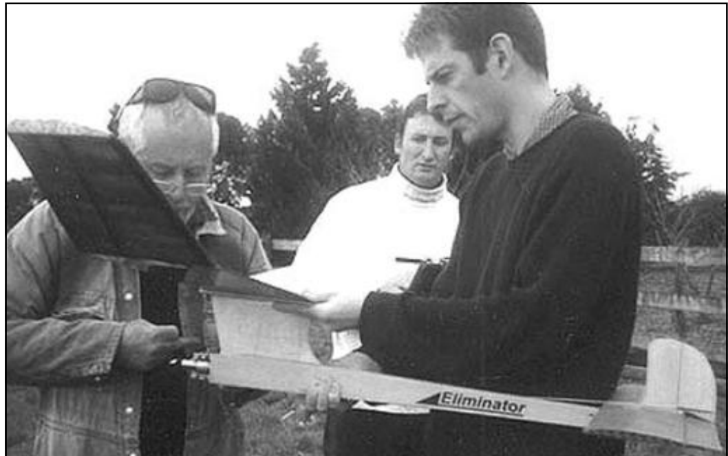
Trevor Boundy, erstwhile WebMaster of SAM 600 Australia, starts his Gordon Burford model "Eliminator" before its test flight. "Eliminator", 50 inch span, Burford plain bearing 2.5cc diesel. Wings covered with SAMspan on top, Mylar sprayed black inside under.
