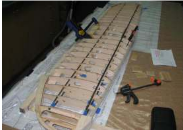
Laser cut ribs with carbon fibre spars. I hate cutting ribs so I bought a short kit from Bellaire in the UK.
