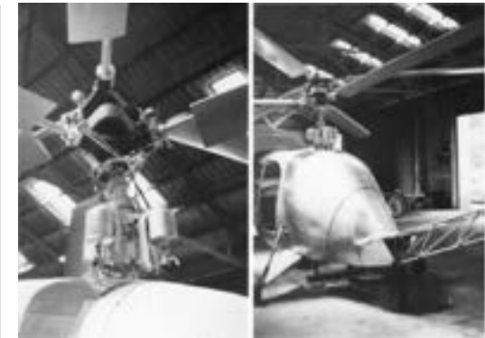
Close up of the contra-rotating prop head and a port rear view of the helicopter.
