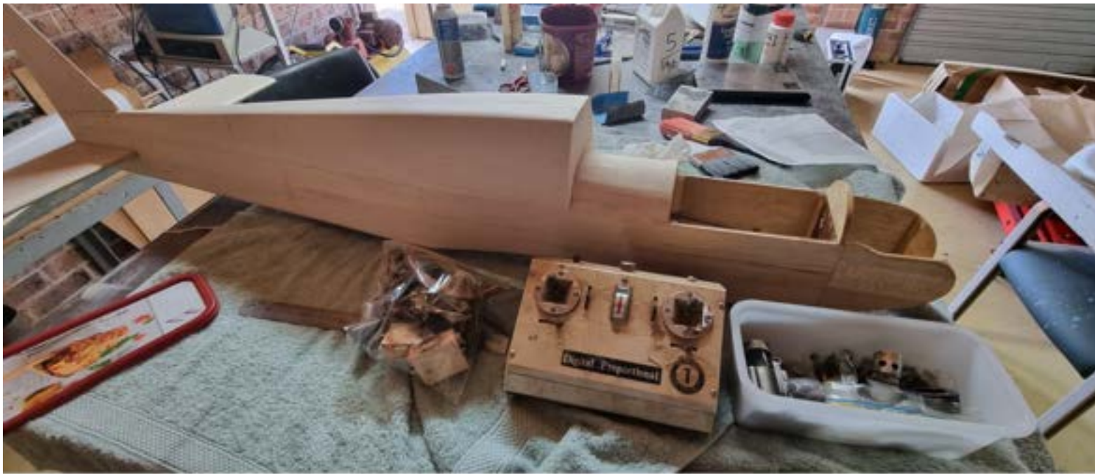
Above: The new Bar-Fli fuselage with the original radio and Merco 61 in tray. Below and right: Original Bar-Fli fuselage and plan, wing and tail.
