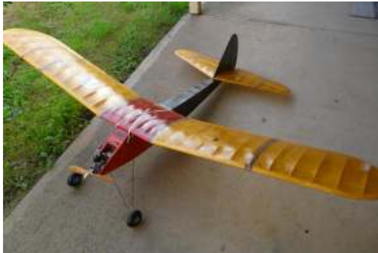
Max Newcombe - Don's Lanzo RC-1 fitted with a Fleetwind 60 Sparkie and scheduled for a full re-cover job in near future.
