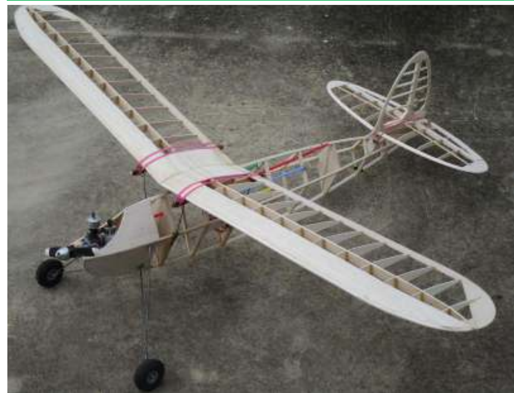
Basil Healy's T-Beam Gas Model in bare-bones form. Power ED Competition Special diesel. Basil entered the finished T-Beam in '38 Antique but engine problems on the start line resulted in a DNS for Basil. Engine now in workshop for new piston.
