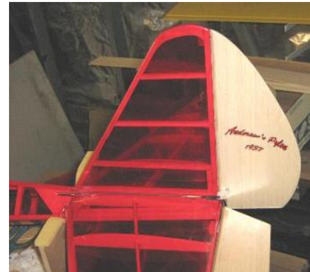
Left: Rear fuse in jig ready for tail mount . Right: Fin Mount to Tailplane with cap strips fitted - lower plates not fitted yet. Below: Completed tail assembly - note foam strip on lower jig plate. Bottom: Pylon plate on fuse - hardwood mounts for servo tray 2nd bay from right
