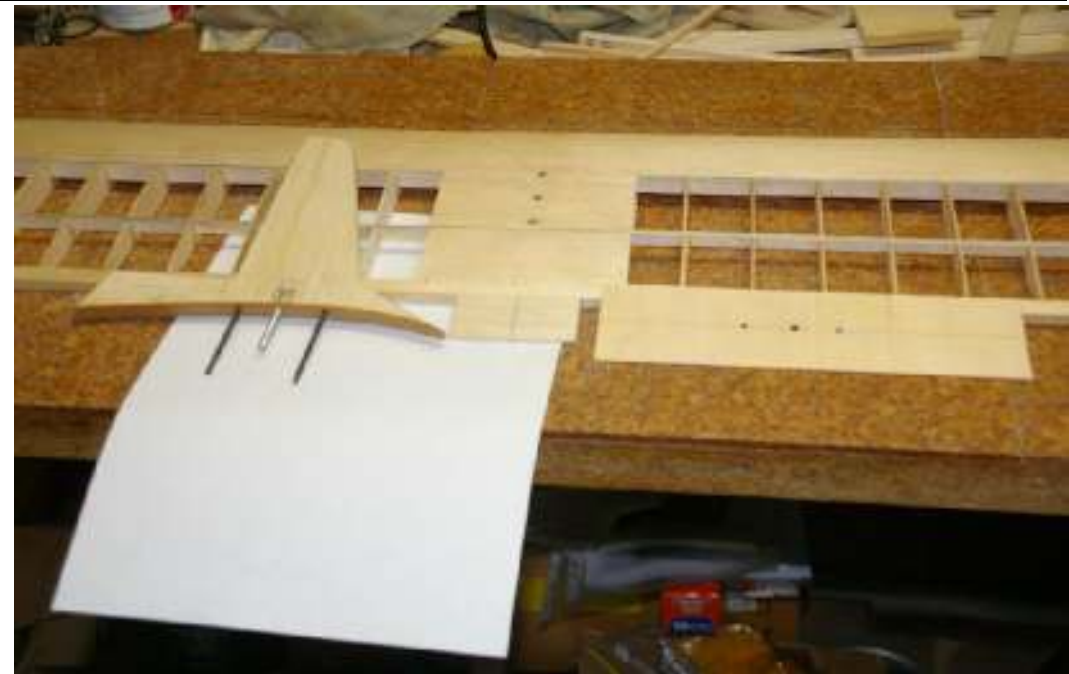
Showing rudder, tailplane and tailplane mount drilled accommodate the removal process.
