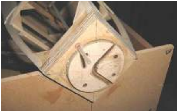
Above: Pylon without top plate in position. Below: Front bulkhead & mount (Fuse on its right side). Plastic tube for throttle push wire. Bottom: Servo Tray (green tube is for antenna wire exit through pylon mounting plate)
