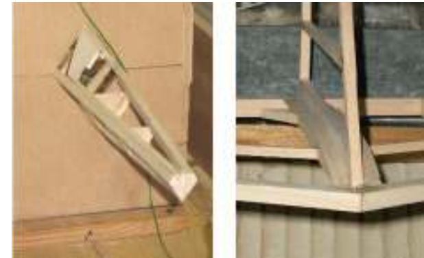
Left: Rear fuse in jig ready for tail mount . Right: Fin Mount to Tailplane with cap strips fitted - lower plates not fitted yet. Below: Completed tail assembly - note foam strip on lower jig plate. Bottom: Pylon plate on fuse - hardwood mounts for servo tray 2nd bay from right
