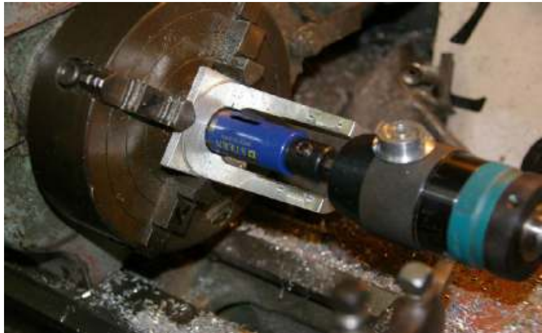
Using a hole saw to remove the centre for weight reduction and to allow access for fuel tank outlet and vent.
