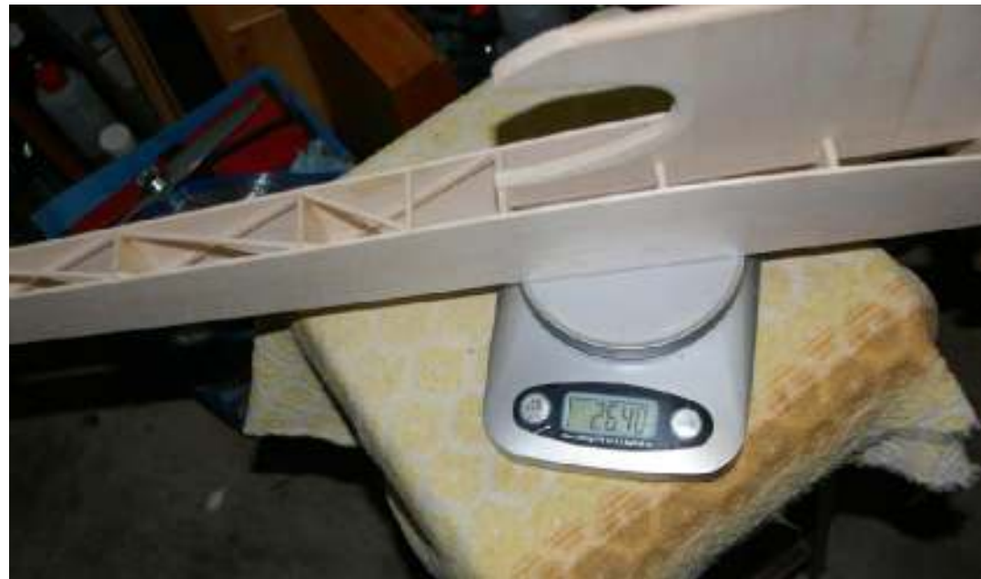
26.40zs so far, also note Warren truss addition to sheeted fuselage, did not add a lot of weight, but increased torsional strength considerably.
