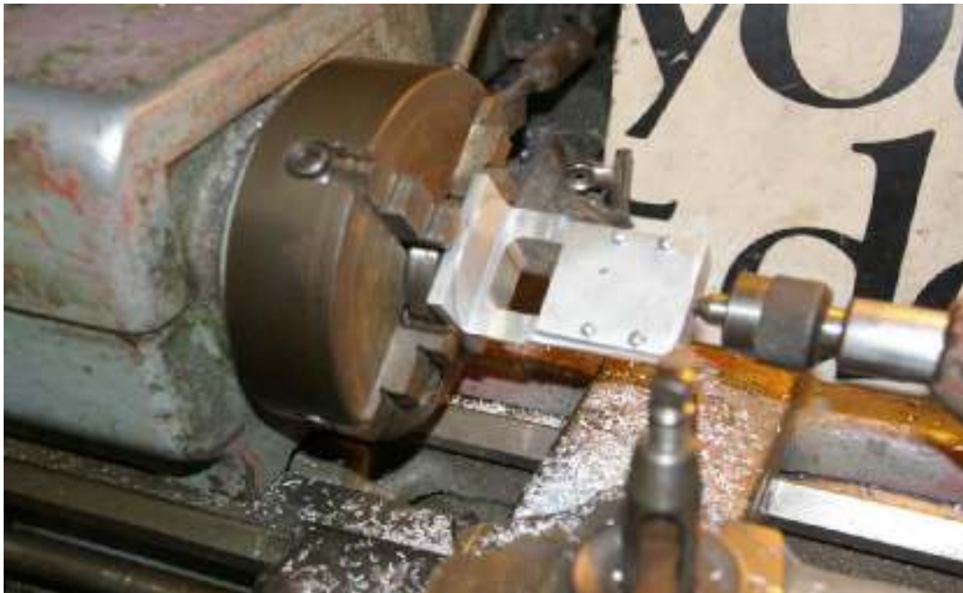
Engine mount set up to remove some weight and to closer fit the mounting lugs.
