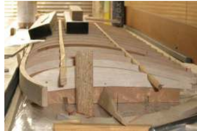
Setting up the wingtip - supports used for wingtip upper spars (basically shortened centre ribs)
