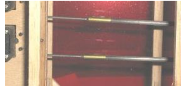
Tube on Carbon rods to prevent rod splitting.
