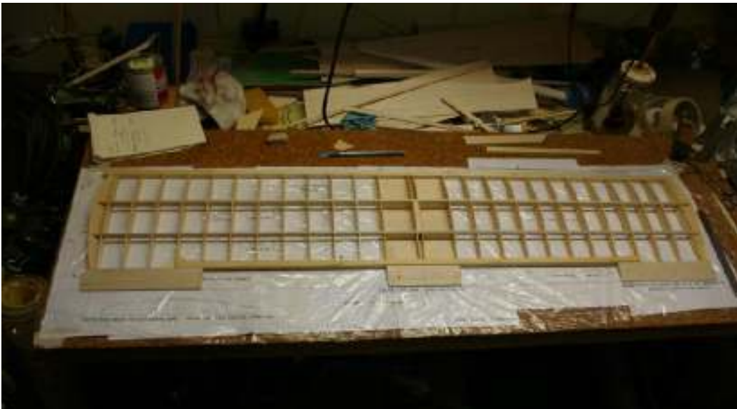
Tailplane under construction.
