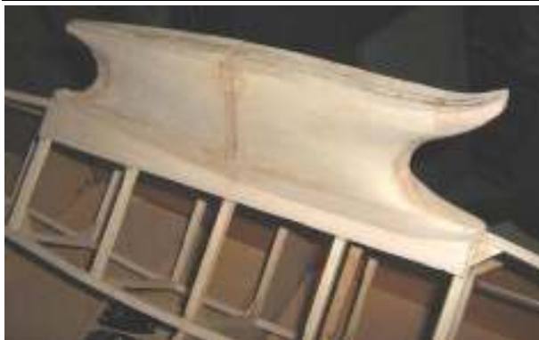
Above: Pylon without top plate in position. Below: Front bulkhead & mount (Fuse on its right side). Plastic tube for throttle push wire. Bottom: Servo Tray (green tube is for antenna wire exit through pylon mounting plate)
