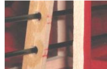
Pushrod support after mating.
