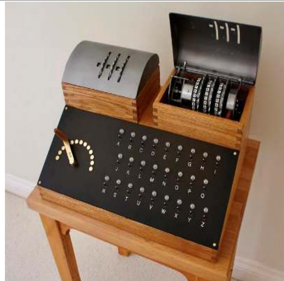
The modern-day cyclometer is about the same size as a very big laptop, but much heavier, with ten kilograms worth of wires, switches and rotors.
