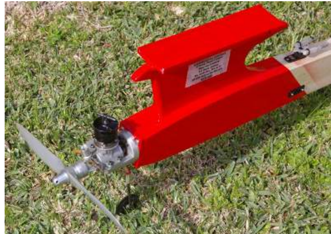
BR Series 13 installed with new engine mount.
