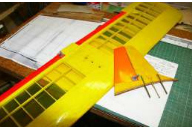
Carbon rods and fastening bolt for fin and tailplane.
