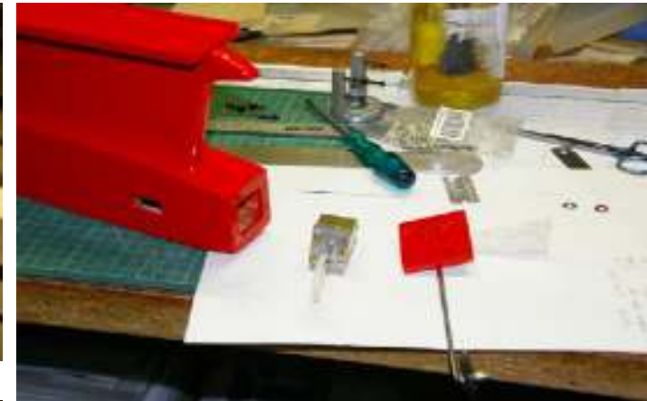
Fuel tank with flanges, firewall, landing leg & engine mount at top.
