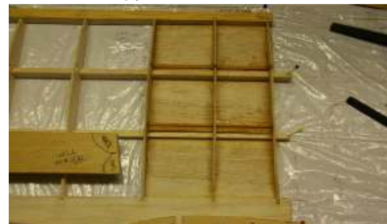
Shows bottom rails epoxied in place.
