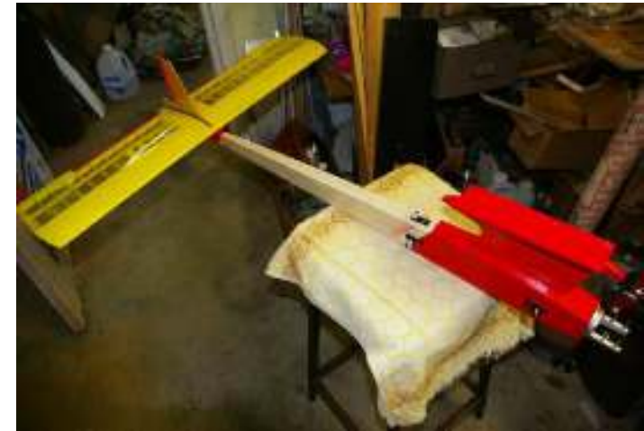
Showing tailplane and rudder assembled to fuselage.
