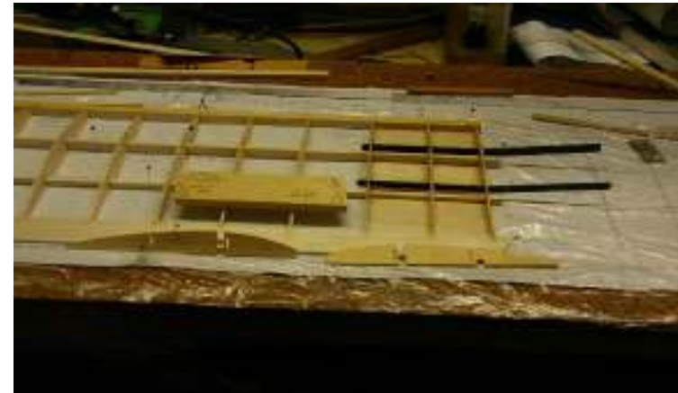
Wing joiners installed into ribs.
