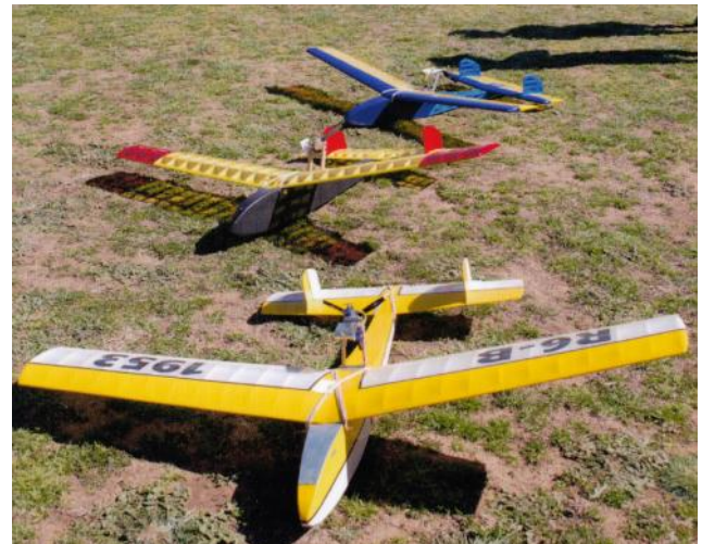
Nominated R/C model for this year's Oily Hand - 60 inch span, R6-B twin fin powered glider with radio by Allan Rowe, New Zealand. Published 1953 Aero Modeller. Only 3 models at Oily Hand. P.A.W. 1.49cc diesels mainly used.
