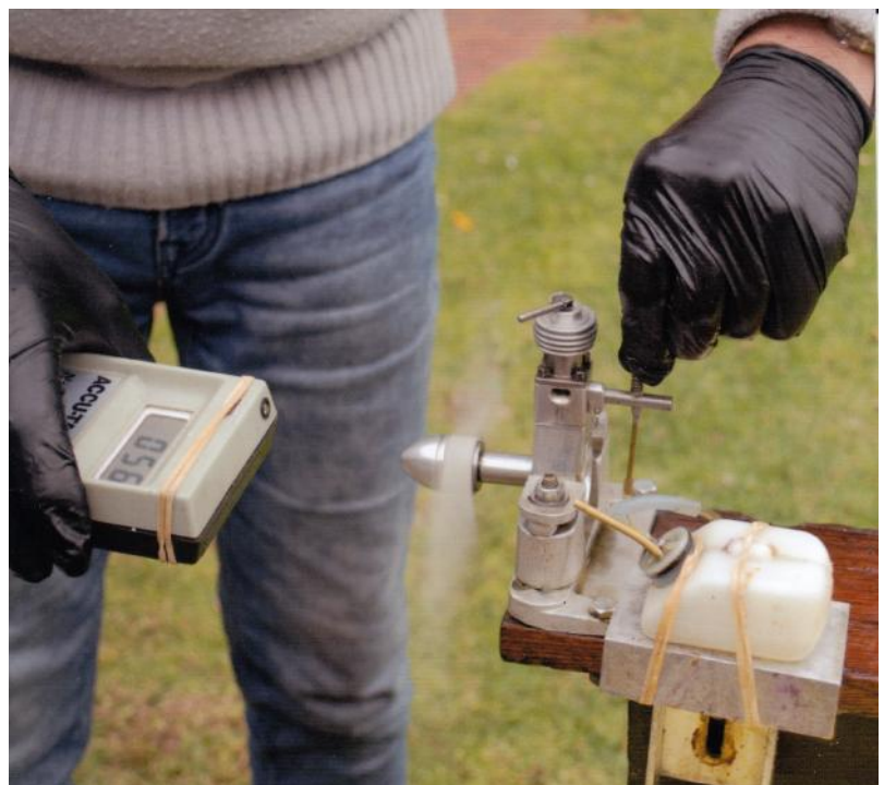
World's first popular diesel model engine, 2.01cc Dyno, introduced August 1941, made in Switzerland. Running on 10x6 Taipan prop, tacho shows 5,600 revs.
