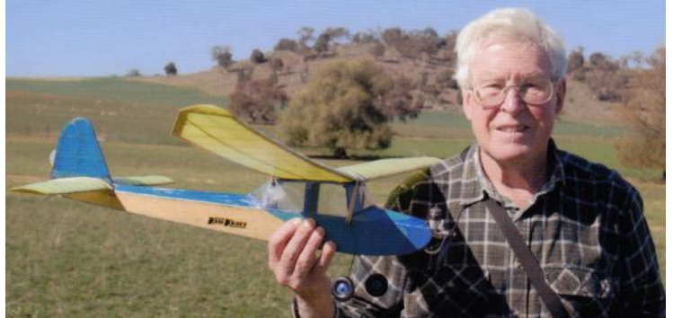
Don Howie (Adelaide) with 1961 KeilKraft "Snipe". Wenmac .449 glo, 6x3 black Cox prop. FF Airspan wings, tail and blue enamel. Over 50 years old. Recovered wings, tail, fin and top of fuselage.
