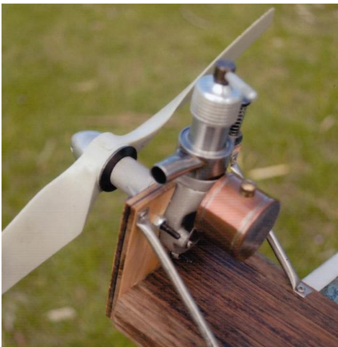
ETHA 2.5cc replica, world's first diesel model engine from Switzerland. Note rear copper tank. Taipan 10x6 prop. Engine No.10 (replica).
