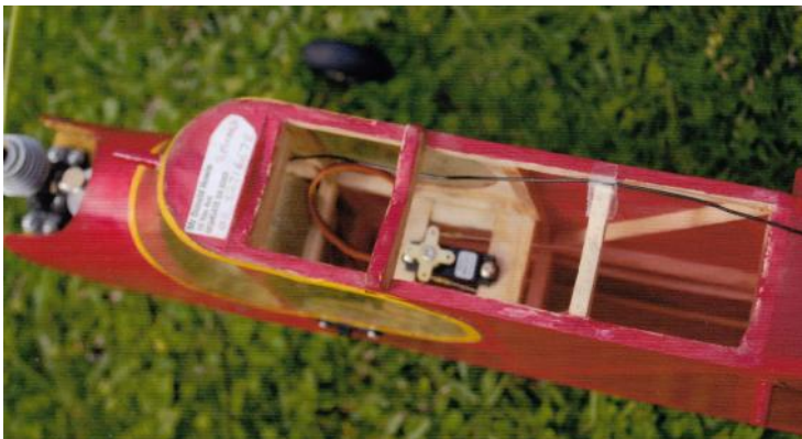
Peter Leaney holds own build F/F "Request" by Frank Ehling. 1941 design published in September 1941 Air Trails magazine. Original model had Bantam .199 spark engine. Peter used a P.A.W. 0.55cc diesel.
