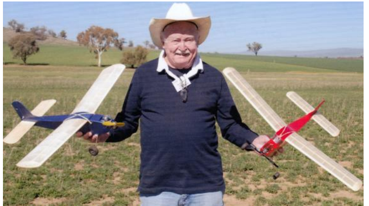
Peter Jackson with R/C assist (emergency use only). Left: "Young Thunder" a design from Argentina P.A.W 55 diesel, silkspan on wing, tail. Tissue and blue paint fuselage and fin. Right: Vic Smeed designed "Popett" 32inch span, Redfin Millish .030 (1/2cc) diesel. Silkspan on wings, tail, tissue and red paint.
