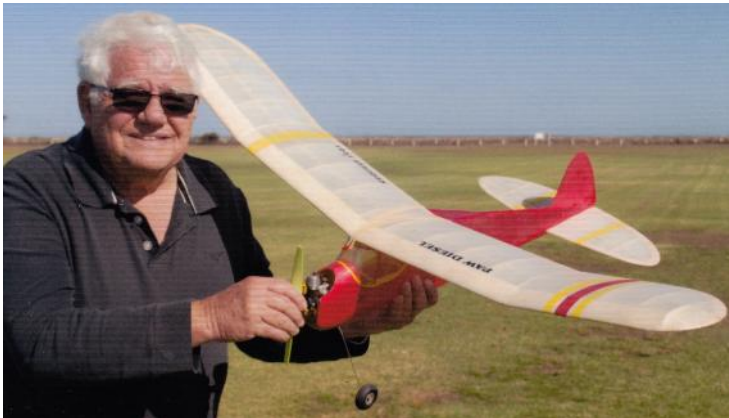
Peter Leaney holds own build F/F "Request" by Frank Ehling. 1941 design published in September 1941 Air Trails magazine. Original model had Bantam .199 spark engine. Peter used a P.A.W. 0.55cc diesel.
