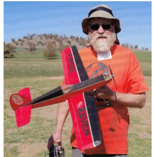
Warren Brown, Mt. Evelyn, Vic. with his double-size (36" span) "Raven" - Frog Senior Series 1953 rubber models (semi-scale 18" span). Engine Oliver Tiger (UK) 0.5cc by Clint Hill Engineering, made by John Ridley. All Airspan covering, two channel R/C ailerons and elevator.
