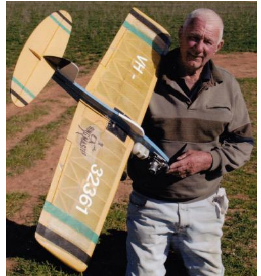
R/C Ringmaster by Geoff Potter. Matt Kania 1951 C/L design for Sterling Models, USA. OS Max 35 glo converted to diesel.
