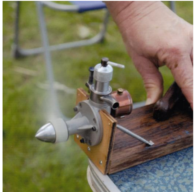
ETHA 2.5cc replica made in 2007 by Richard Gron, Czech Republic. Engine running on 10x6 Taipan prop. Note front, large radial mount.
