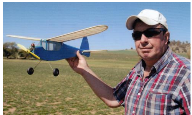
Vic Smeed "Courtesan" by Ian Le Bronne. 26" span Tissue on wings and tail. D.C. Dart 0.55cc diesel.
