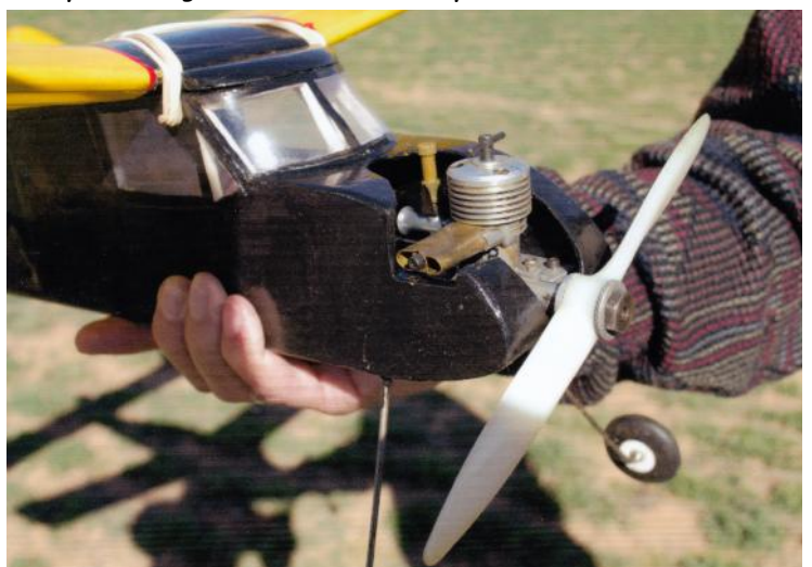
Above: Black and Yellow fifties design "Apex" by Mike Minty. E.D. Cadet 0.98cc (1cc) diesel, 8x4 prop. Note home made muffler.
