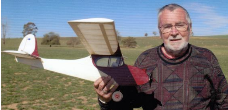
Mike Minty (Sydney) and his "Cricket" design by Noel Shennan from Model News magazine (Australia) R/C Assist. C.S. Redfin 0.8cc diesel 8x4 prop. Polyspan covering and paint.
