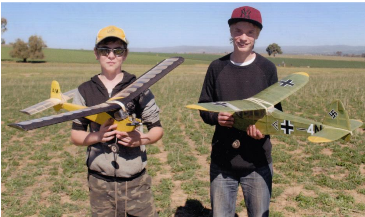
Warren Brown, Mt. Evelyn, Vic. with his double-size (36" span) "Raven" - Frog Senior Series 1953 rubber models (semi-scale 18" span). Engine Oliver Tiger (UK) 0.5cc by Clint Hill Engineering, made by John Ridley. All Airspan covering, two channel R/C ailerons and elevator.
