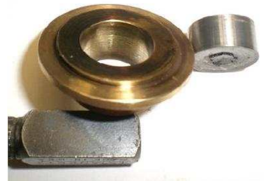
Here is the button which contains the contra-piston under the cylinder head. In this picture the contra-piston has been removed.
