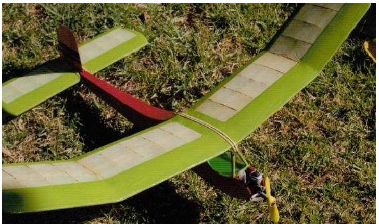
Canowindra SAM 1788 Champs, Brad Turner with his "Fright", K&B 40 rear intake F1 pylon engine with Dubb Jet muffler. Covered with laminate film and Hobby King covering.
