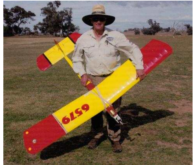
Peter Van de Waterbeemd with "Schmaedig Stick", GB 5cc Mk.1 diesel, 13½x6 Bolly Clubman prop, Hobby King covering.
