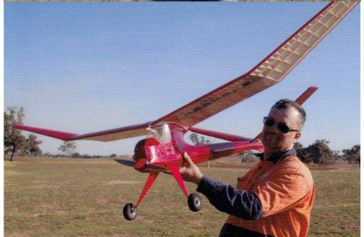
Canowindra SAM 1788 Champs, Brad Turner with his "Fright", K&B 40 rear intake F1 pylon engine with Dubb Jet muffler. Covered with laminate film and Hobby King covering.
