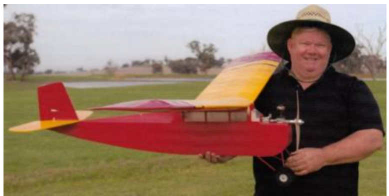
Canowindra 2017 SAM 1788 Champs. Anthony Vicary from Narrandera NSW with his Trenton Terror / ED 346 Hunter diesel. Solarfilm on wings and tail. Polyspan and paint on fuselage and fin.
