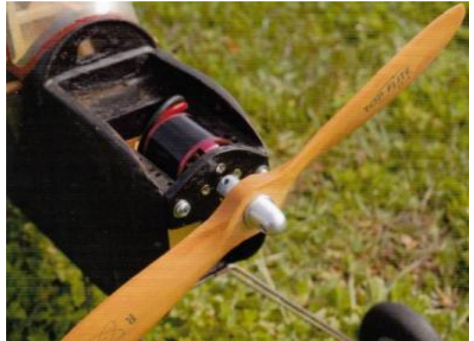
Mounting plate shown to convert "Trenton Terror" to electric power. 12x5 TopFlite wooden prop.
