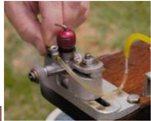
McCoy .049 Diesel with Poppet Valve running nicely.
