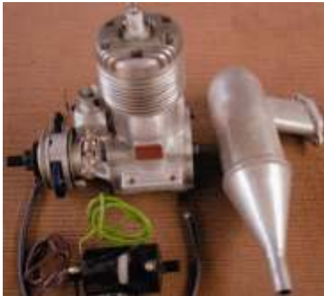
SAITO G 60 F two-stroke, spark engine. Released 1975 with coil, muffer etc. Also came as rear-induction version. Below: The other side. Has markings for start/run arm position on spark timer.
