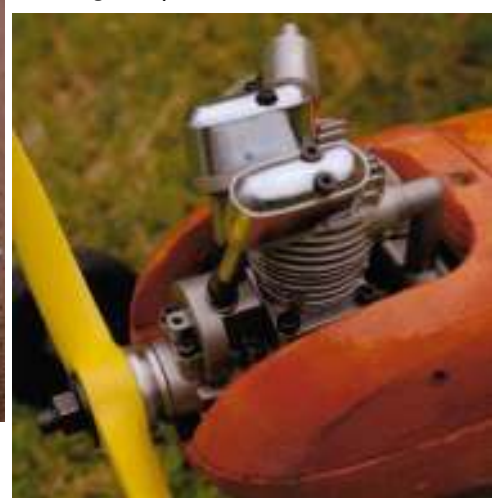
McCoy .049 Diesel with Poppet Valve running nicely.
