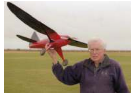
Don Howie holds 48 inch span Scarlet Tanager, 1938 Plan. Electric Powered 8x6, electric prop, 2 cells 1500 mah 2S.
