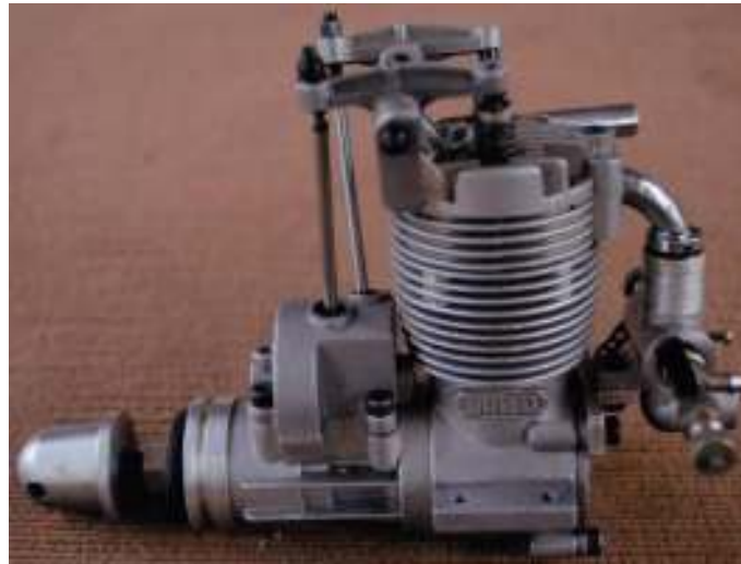
First SAITO F.A. 30 four-stroke engine, 1979, owned by Bill Britcher. At Right: Recent SAITO F.A. 30 (5cc). Great running engine. 11x4 nylon prop.
