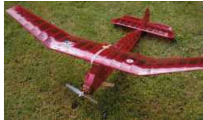
1/2A Texaco "Red Ripper" converted to electric 1/2A. Turns Taipan 7x4 prop. Colour matches name of model. 460 mah 2S lipos fitted. Flown by Don Howie.
