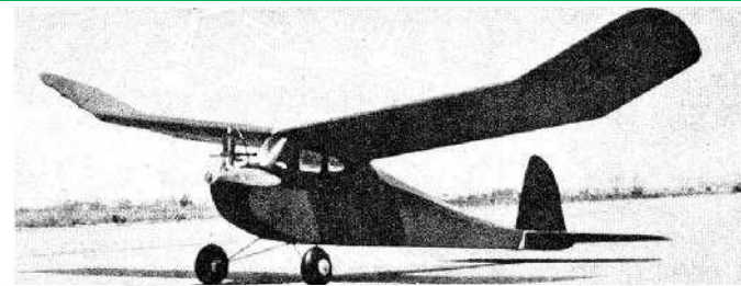
Bombshell was Brown-powered. Fuselage had sheet sides, formers, stringered turtlebacks.
