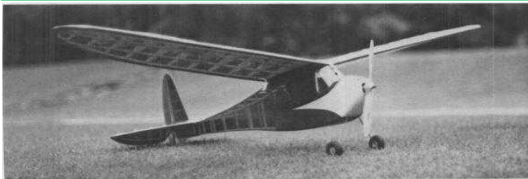
Nice thing about transparent covering, whether it's silk and clear dope or see-thru film, you can still see that pretty framework . . . something you can't get with foam and fiberglass.
