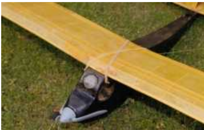
Test aircraft - 1/2A ATOMIZER with Speed 400 motor and 6x3 Graupner folding prop.
