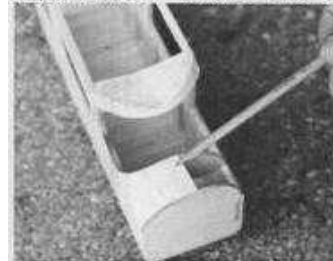
Curved portion of cowl after wet forming.
