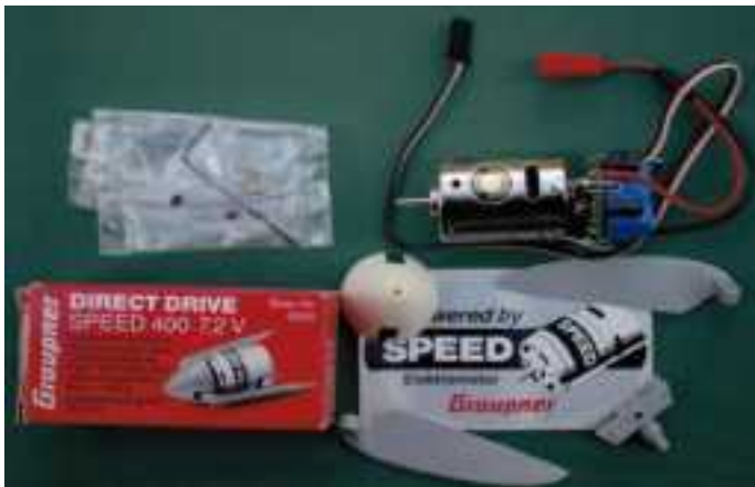
Left: Speed 400 Pack by Graupner includes flux lux ring and 6x3 folding prop. Right: Mabuchi 380 pm motor with Robbe switch, B.E.C., brake fitted. Also parts for 6x3
