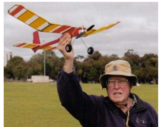
Don Howie with 30" span modified "Presto" design by Maris Dislers powered by Arne Hende replica Elfin 50 diesel.
