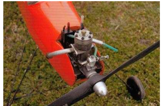
ASP 40 Glo converted by Geoff Potter to diesel with small Enya carburettor in Rex Brown's Flamingo.
