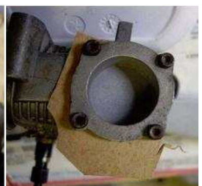
Fit screws carefully cut away surplus
