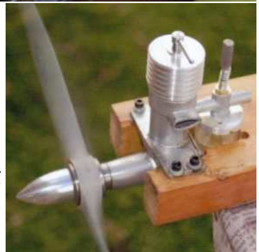
Left: Mystery Engine. Suspect it was made by John L. Doll who was an aeronautical engineer. He designed the early "Syncro" engines. Radial mounting shown.
