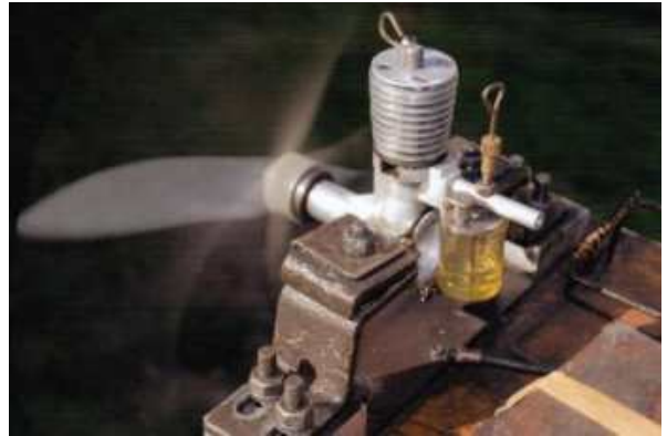
C.I.E. diesel, 2.4cc, from Modelcraft, California. 1947 model by Hy-Pro, Barney Snyder Company.
