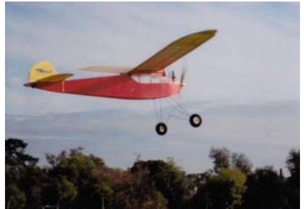
48 inch Heron (Gas Buggy) flying in Adelaide West Parklands. Has American A.H.C. diesel up front.
