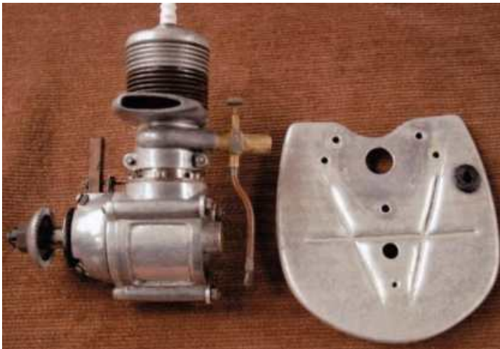
Above Right: Gordon Burford made 2cc "Deezil" (copy of original from 1948). Starts and runs easily. Engine owned by Bill Britcher.
