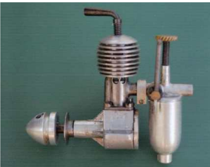
1948 2 nd model "K" Hawk 0.24cc diesel. Smallest British engine in the nineteen forties.
