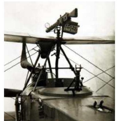
This early German AEG two-seater has a Parabellum machine gun mounted to swivel forward at an angle. Note the wire guards to prevent firing into the propeller arc.
