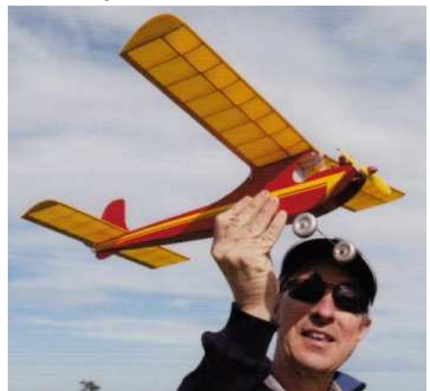
Oily Hand Weekend - Maris Dislers (S.A.) 24inch span Veron Cardinal (original 35inch span) Clan 0.24cc diesel
