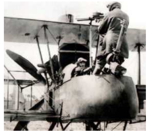
The British Fe2b "pusher" biplane had a rear-mounted engine, which was awkward, but in the early days it provided the best option in forward-firing guns.
