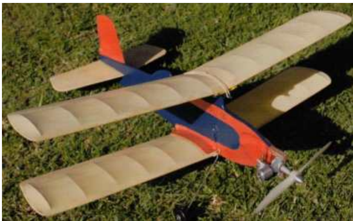
23inch span Fli-Bi by Don Howie, 7½oz, replica 0.4cc Micro Diesel cream air span on wings and tail, Humbrol paint on fuse and fin.
