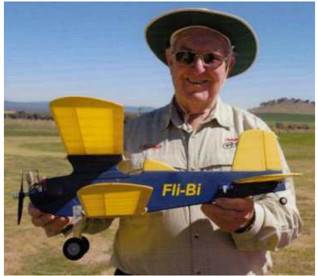
Oily Hand Weekend - Cowra, Sat. 26th August, 2017. Alan Wooster 28inch span R/C Fli Bi MP Jet 0.6cc Classic Diesel.
