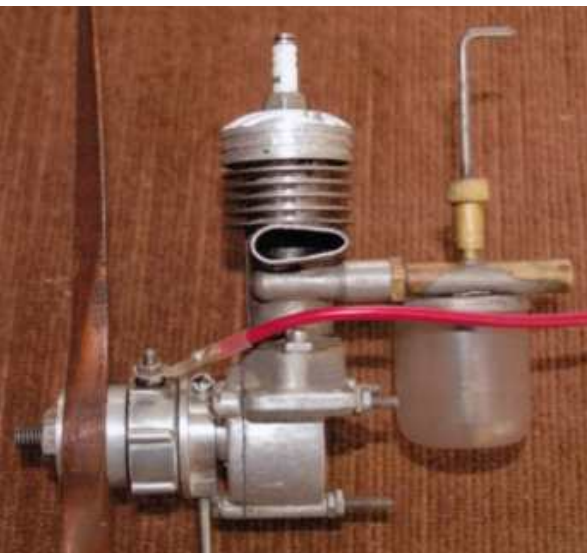
Below: 1939 Madewell .147 cubic inch Spark engine fitted with modified McCoy timer. Made by Jack Keener and Jim Brown, Oaklands, California. USA.
