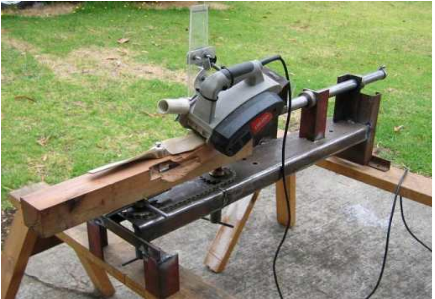
Another of our projects was a propeller blank cutter.
