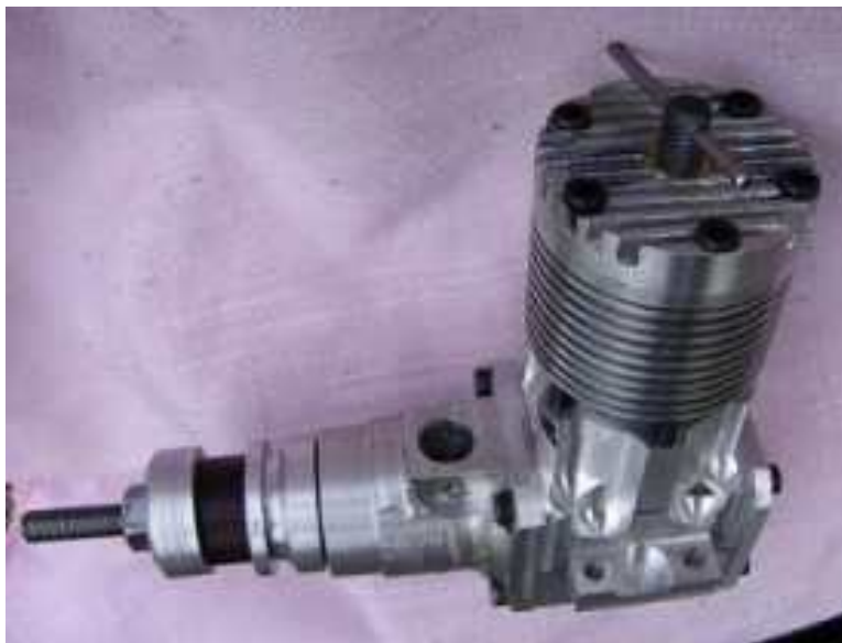
Trevor's 40 Diesel, (now sitting atop of the Stebbing Memorial Trophy) showing external machining and the bushed compression screw in the head.
