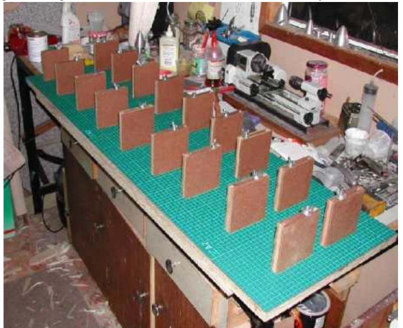
Figure 6: Jig blocks loosened on one side so that formers may be removed.
