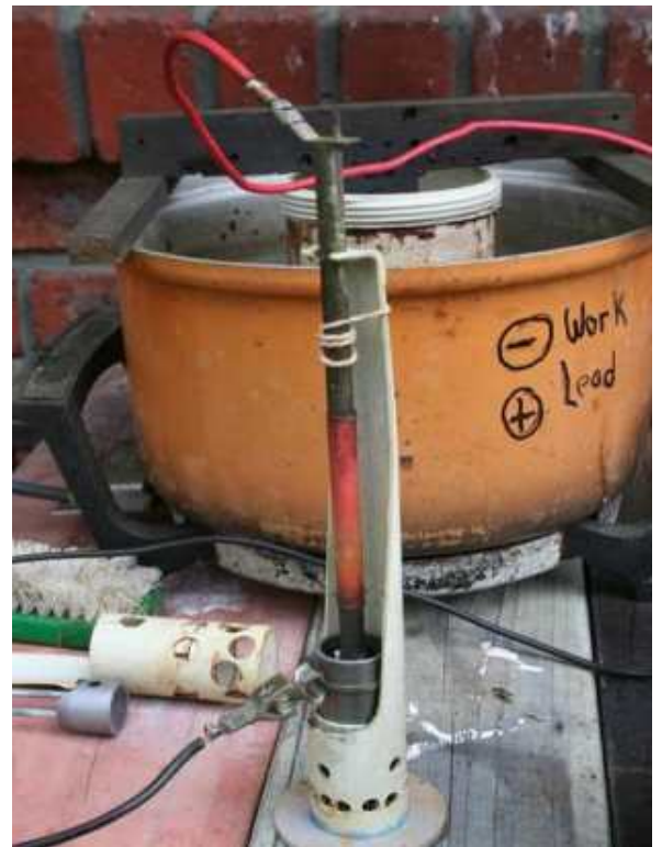
Above: Chrome plating at Trevor's, showing work holder and temperature controlled plating bath made from chip fryer.
