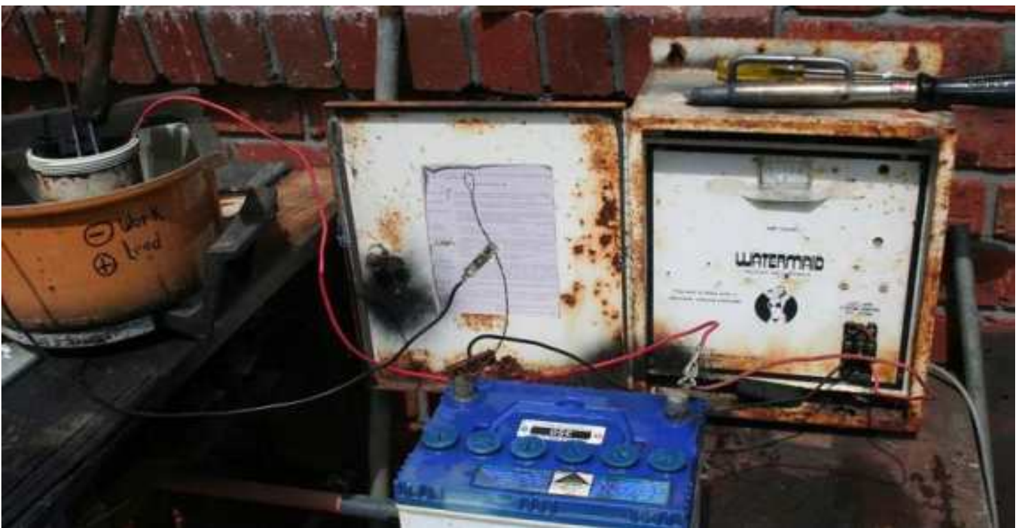
Below: DC power supply using 12 volt DC swimming pool chlorinator and car battery.
