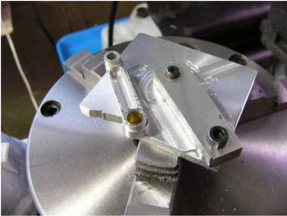
Milling jig for machining the bushed con rods.
