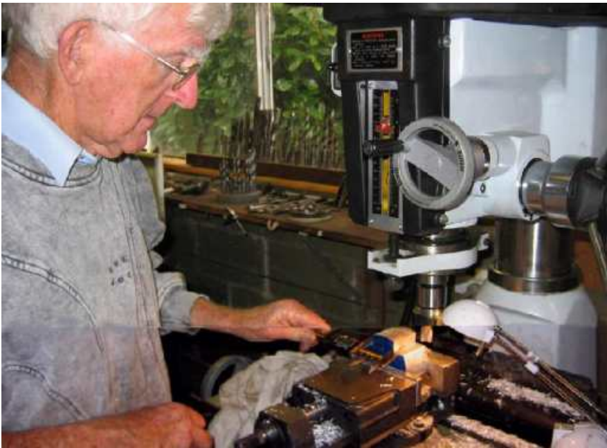
Milling jig for machining the bushed con rods.
