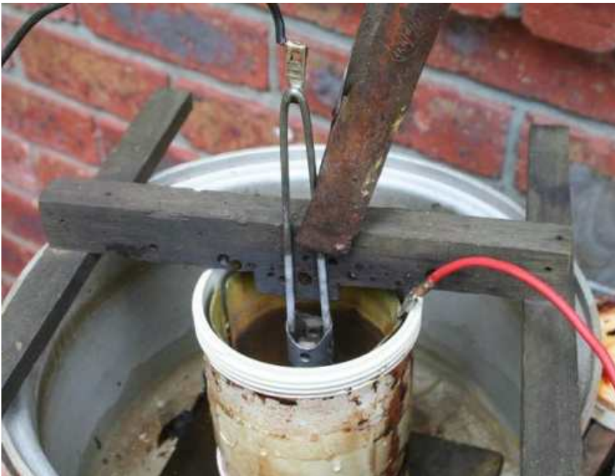
Above: Chrome plating at Trevor's, showing work holder and temperature controlled plating bath made from chip fryer.
