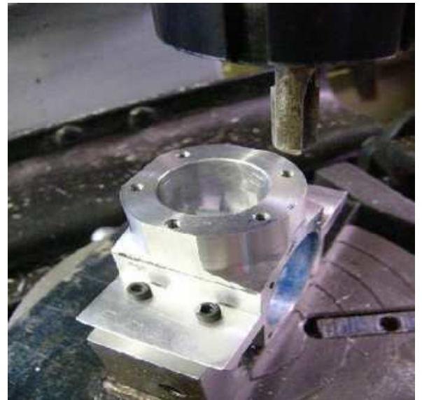
40 diesel start of crankcase on Fred's new mill 2005 March.
