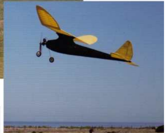
Below: Forster 99 sparkie in Bill Britcher's "Anderson Pylon" the first pylon model by Alva Anderson in 1937. The original had a Forster 99. 16x10 wood prop hand-carved by the late Max Starick.
