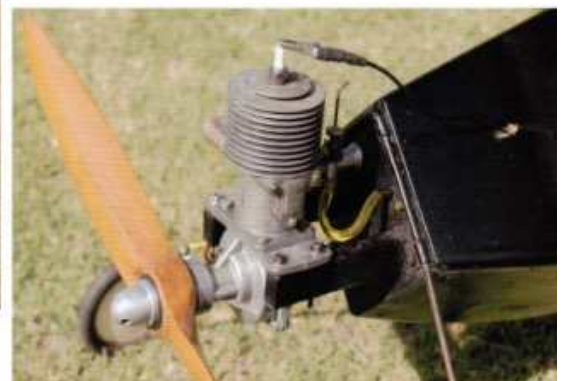
Below: Forster 99 sparkie in Bill Britcher's "Anderson Pylon" the first pylon model by Alva Anderson in 1937. The original had a Forster 99. 16x10 wood prop hand-carved by the late Max Starick.
